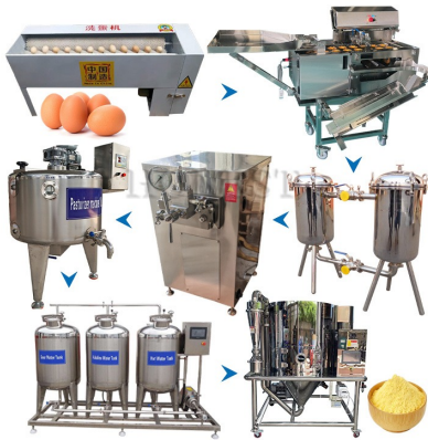
Made-in-China supplier reference: real egg washing, breaking, filtration, pasteurization, CIP and spray-drying line.
