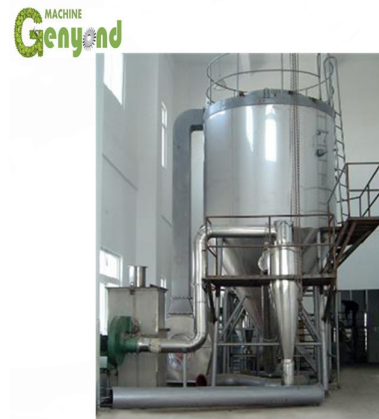
Made-in-China supplier reference: real industrial spray-drying tower used for egg powder.
