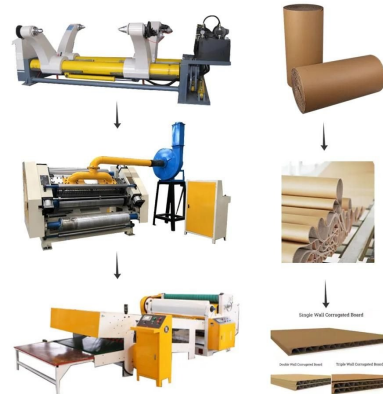
Made-in-China supplier reference: second real machine configuration for two-ply corrugated-board single-facer line.
