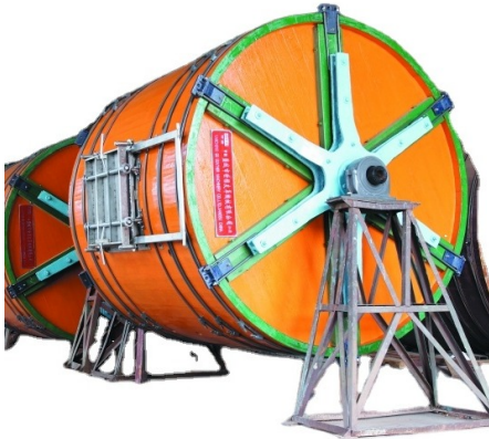
Alibaba supplier reference: real wooden process drum used in hide soaking, tanning and dyeing.
