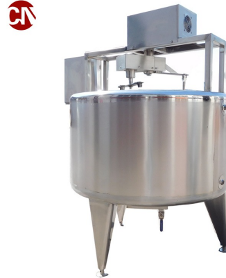
Made-in-China supplier reference: real jacketed stainless cheese vat with curd cutting and agitation.
