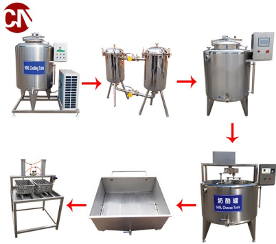
Made-in-China supplier reference: real small white-cheese process with cooling, pasteurizing, cheese vat, drainage and press.
