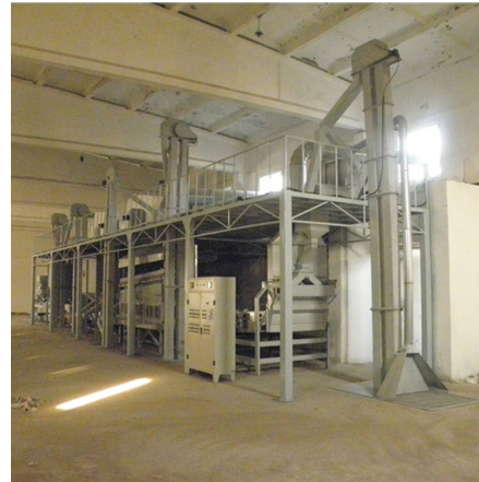
Supplier reference: modular wheat-cleaning and grading plant with elevators.
