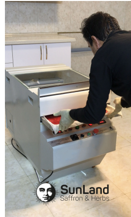
Processor reference: real controlled saffron tray dryer used to protect color and aroma during moisture correction.
