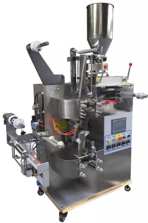
Made-in-China supplier reference: real inner-and-outer herbal tea-bag packing machine.
