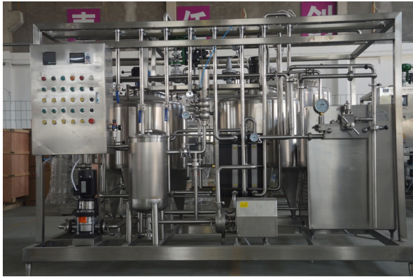
Made-in-China supplier reference: real small dairy/beverage processing line with mixing, heat treatment and sanitary tanks.
