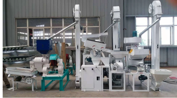
Supplier reference: real one-tonne-per-hour rice milling and polishing equipment arranged as a compact line.
