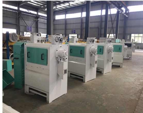
Supplier reference: dedicated barley peeling and pearling machines photographed in the manufacturer's workshop.
