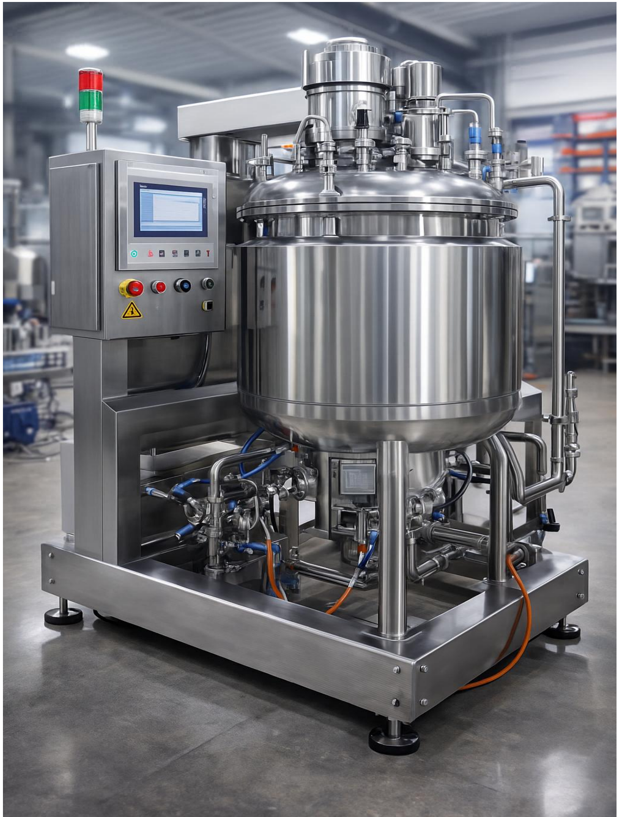
Vacuum mixing tank used for premixing and homogenisation
