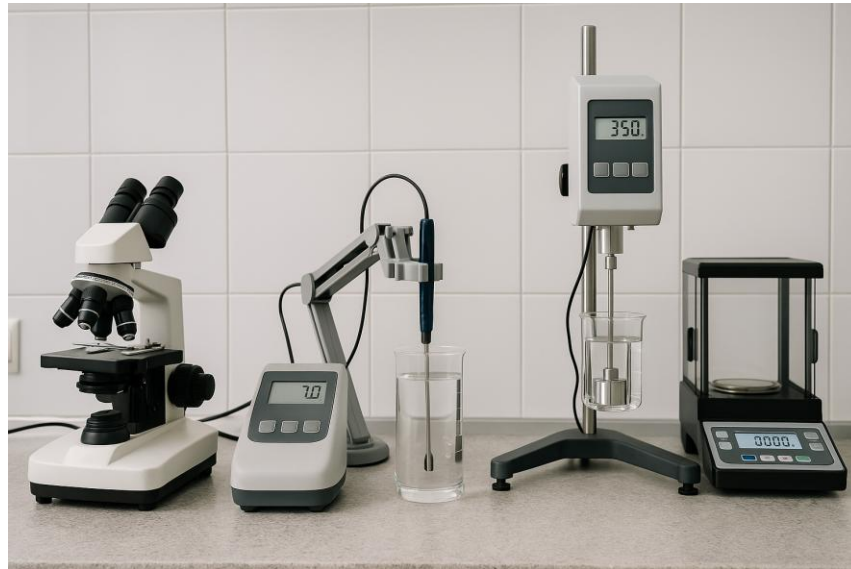
Quality control laboratory with pH meter, viscometer and microscope
