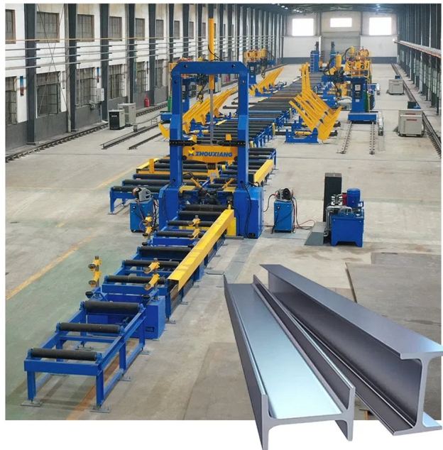
Automatic H-beam cutting, assembly and welding line
