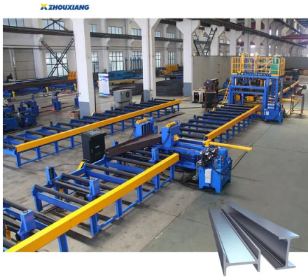
Horizontal automated beam fabrication line
