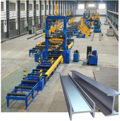
Automatic H-beam cutting, assembly and welding line
