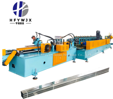
Made-in-China supplier reference: real metal studs & drywall channels production line equipment.
